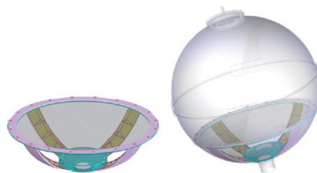
图 1 月球着陆和上升器 \text{LO}_2/\text{LCH}_4 贮箱 PMD 方案 Fig. 1 Lunar descent stage RCS and ascent stage RCS/ME tank partial PMD
