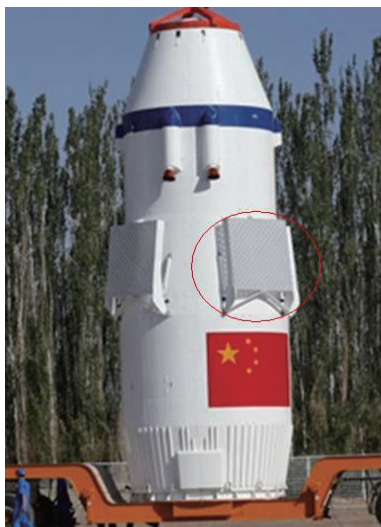
图1 CZ-2F逃逸飞行器应用栅格翼作为稳定翼面 Fig. 1 The grid fins were adopted as stabilization device for abort vehicle of CZ-2F
