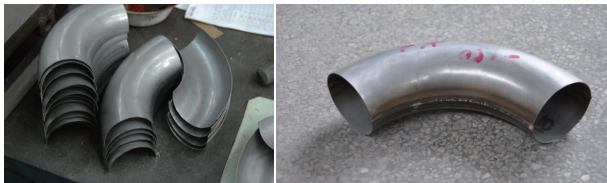
图1 传统拼焊工艺制得的弯管 Fig. 1 Traditional tailor welded elbow
