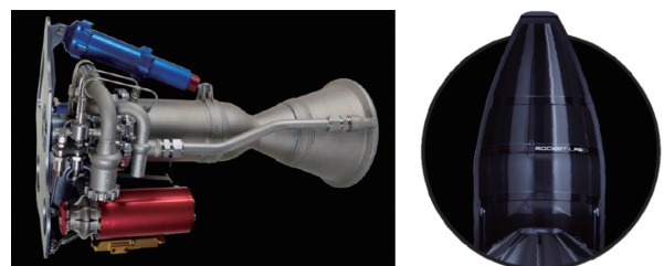
图 2 电子号小火箭的单台发动机和复合材料整流罩 Fig. 2 The single propulsion and composite fairing of Electron small launch vehicles
